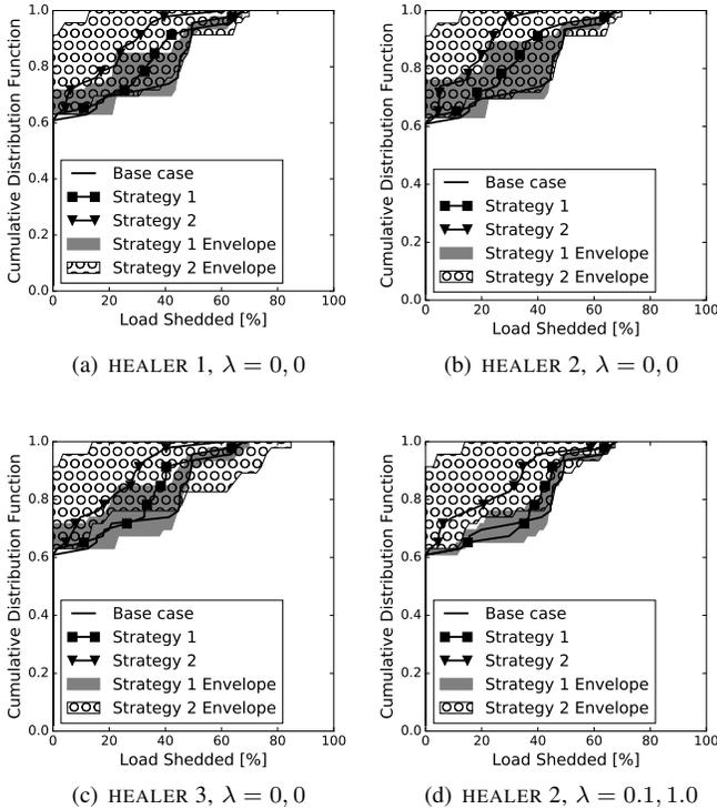
Fig. 2. Load shedded in case-39 with AC power flow under different healing modes and  $\lambda$  values for STRATEGY 1 and STRATEGY 2 respectively.
